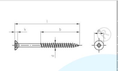
Item 904741 A4 TX **Double CSK head timber screws with** ribs, cutting point
